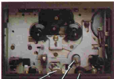
HEADS CAPSTAN ROLLER (turns clockwise)
