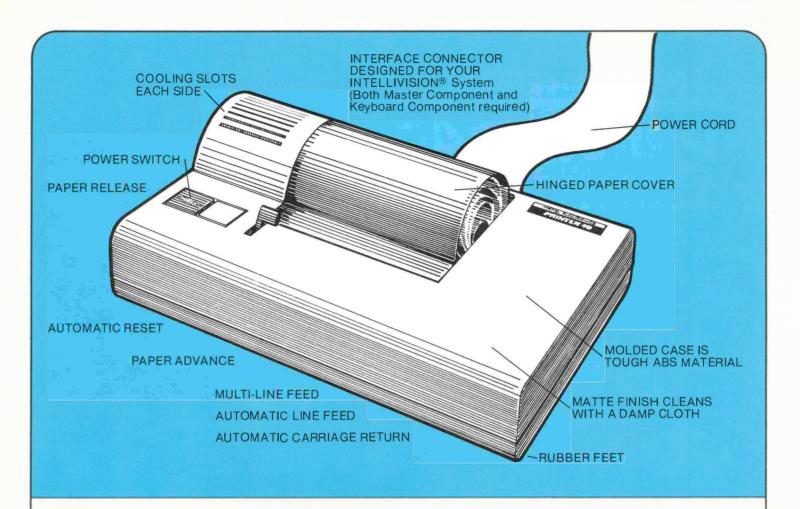
The MATTEL ELECTRONICS PRINTER 40 is a highly reliable printer/plotter that operates with low power consumption and provides long-life expectancy. Connector provided will interface with your INTELLIVISION® Keyboard Component.
